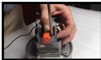
9. Assemble motor after brush replacement: snap plastic fan cover back into place, feed ground wires back through backplate, put housing back on to motor, pull cord set back to normal position, (**make sure wires do not get smashed between metal ring and housing.** fasten ground wires to backplate, turn motor over, tighten flange on top of housing and gasket.
