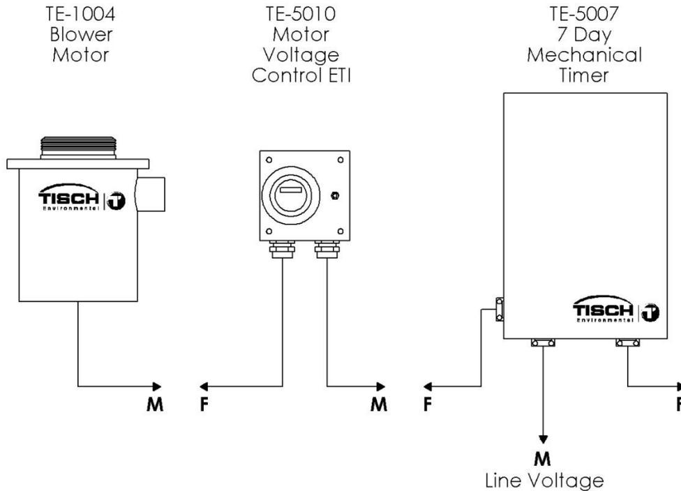
1. The TE-1004 PUF Blower Motor male cord set plugs into the TE-5010 Motor Voltage Control Female cord set.
