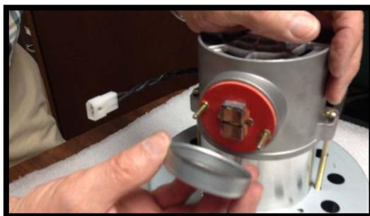
2. Remove the copper brush assembly clips to release the brush and spring assemblies (TE-10542).
