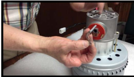
4. Insert new carbon brushes in the brush holders and secure with the four brush assembly clips.
