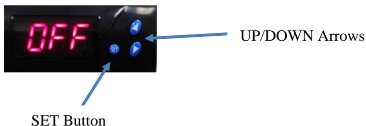
3. Use the UP / DOWN arrows on the timer to change how long the instrument should operate in minutes.
