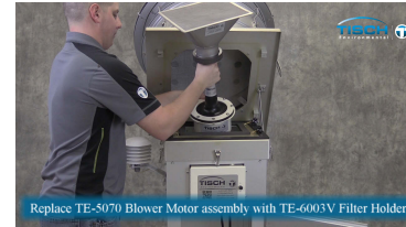
Replace TE-5070 Blower Motor assembly with TE-6003V Filter Holder
