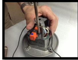
6. Push brush carbon against armature until brush housing falls into brush slot on motor.
