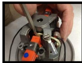
5. Carefully slide quick disconnect tabs into tab slot of new brush.
