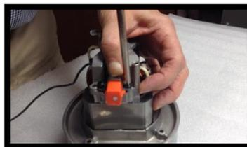
9. Assemble motor after brush replacement by replacing the motor cushion and metal motor ring(s), placing housing over and down on the motor (at same time pull power cord out of housing), being careful not to pinch any motor wires beneath the motor spacer ring.
