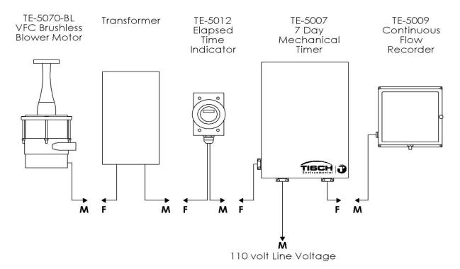
The TE-5070V-BL Brushless Blower Motor male cord set plugs into the Transformer Female cord set.
