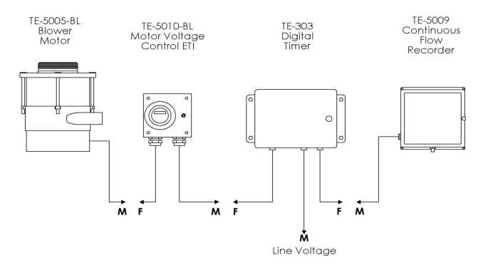
The TE-5005D-BL Blower Motor male cord set plugs into the TE-5010-BL Motor Voltage Control Female cord set.
