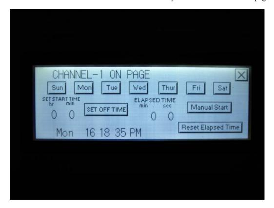
Press the **DAY OF THE WEEK** FOR DAYS THE SAMPLER IS TO RUN.
