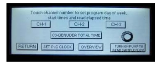
Press **OVERVIEW** button will take you to the overview page. When anything is on or off this page will show you the status of the sampler in the three round lamps and when the pump is on. The set time for each channel is displayed when they are installed.
