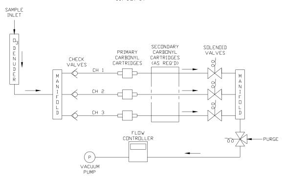
Figure 1. Tisch Aldehyde Sampling System Configuration.
