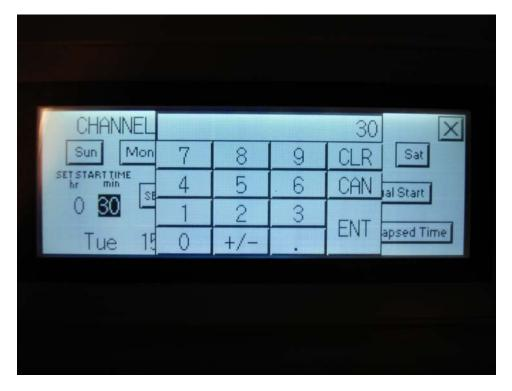
Touch the time you want the sampler to start and touch **ENT** on the menu. If the sampler is to start on an even hour, press 0 and **ENT**.
