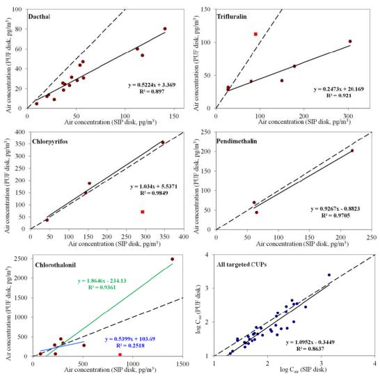
Figure 3. Comparison between SIP and PUF disk samplers using linear regressions of measured air concentrations of CUPs in pg/m³. Red squares show outliers, which were excluded from correlations. Chlorothalonil graph (bottom left panel) shows correlations with and without the highest concentrations. The bottom right panel shows correlations of logarithmic values of air concentrations for all targeted CUPs. The 1:1 dashed line represents perfect agreement.
