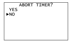
The ABORT TIMER menu (shown above) is displayed when the "F1" soft-menu function key is pressed from the main status display and the timer is currently executing. This allows the user to stop a currently executing timer event and re-configure the timer to the desired settings. Once a timer event is aborted, the timer will not execute until it has been reprogrammed with a valid start time and duration. To stop a timer that has not started use the STOP and EXIT option in the TIMER SETUP menu.
